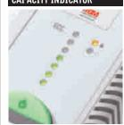
"ECC" (Electronic Capacity Control) indicator helps prevent paper jams by monitoring capacity levels during operation.
